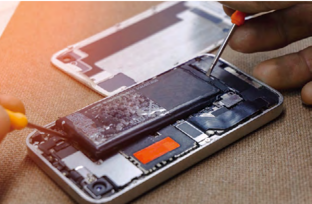
When used to secure mobile phone batteries, electrical release tape allows for quick and easy battery replacement using an electric current.
