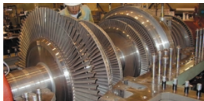
Steam turbine that produces electricity
