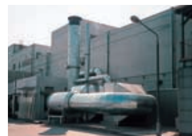
Catalyst deodorizing furnace at Nitto Denko (Shanghai Songjiang) Co., Ltd. (China)
