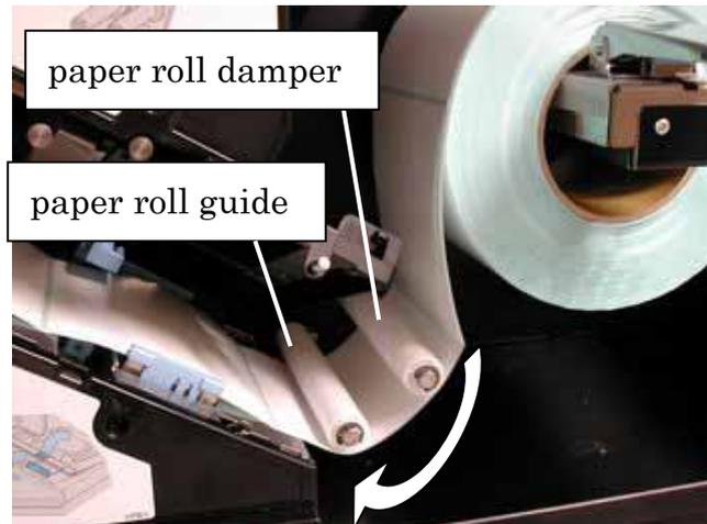
7. When you use a roll wound with labels inside, run the paper over the paper roll damper and under the paper roll guide.
