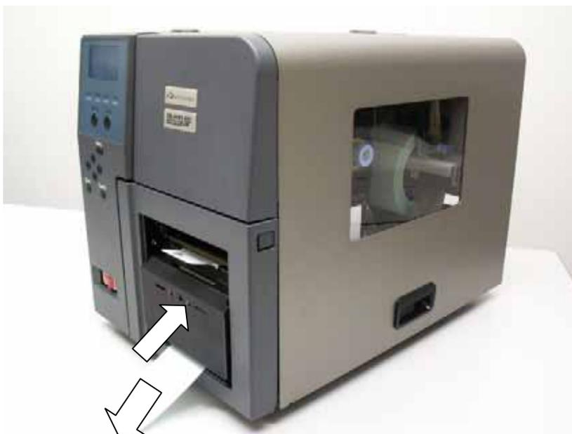
A printed label is peeled off from the backing paper and held on the upper side of the peeler unit. In the case of printing more than one labels, the next label is printed and held similarly after the previous one is taken off.
