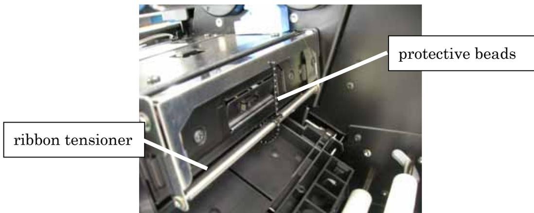
6. Unlock the front cover by pressing the front cover unlock button and pull open the cover.
