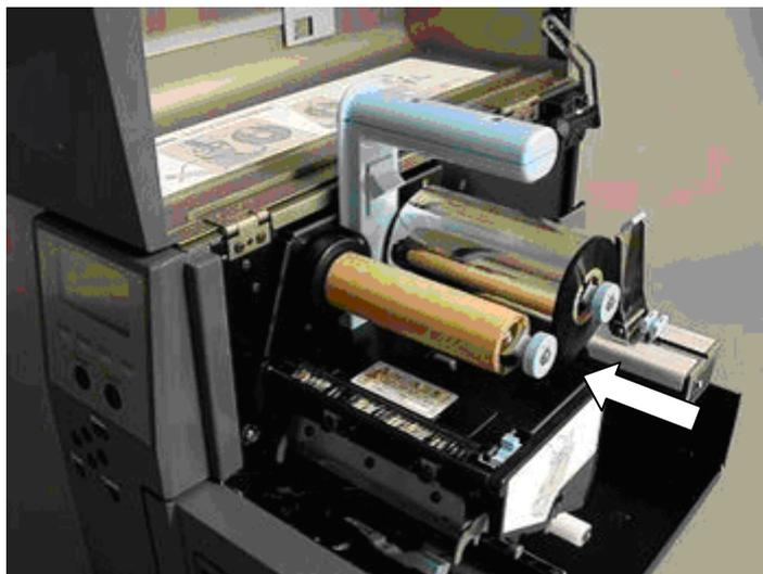
7. Peel the end of the new ribbon off the roll. Pull the ribbon out, run it under the head unit and paste the end of the ribbon (adhesive on it) to the take-up ribbon core.
