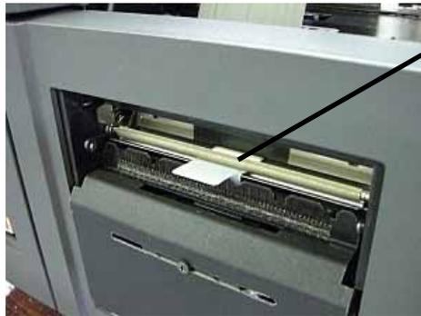
Feed the paper by pressing the “Feed” key and peel the labels outside. You can measure length instead of pressing the “Feed” key.
