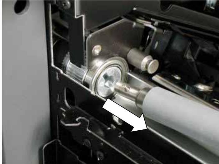
Remove the paper wrapped around the platen roller.
