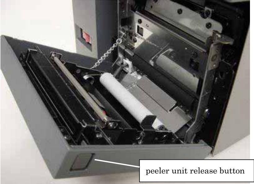
Measure length with the unit closed and without setting labels through the peeler. If you measure length with the labels set through the peeler unit, "Feeding Error" occurs. See to it that the paper of at least 15cm long sticks out of the printer cover when the length measurement is completed. If the length of the sticking paper is less than 15cm, repeat the alignment of print start position until the paper longer than 15cm comes out (when label pitch is small).
