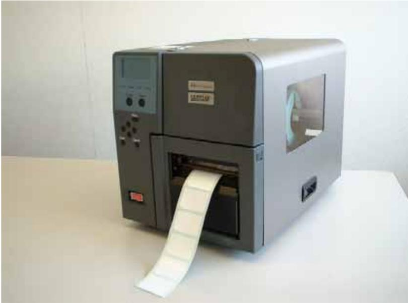
Insert the label-removed backing paper into the slot between the rubber roller (black) and the pinch roller (white).
