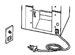
● The AC mains should be capable of providing at least 15A
