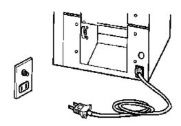
The voltage must be 110V or less at no load (when the printer is not connected), and 90V or more at full load (when the printer is connected and operates).
