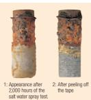
IOS Salt Water Spray Tester Test Time: 2,000h Test Evaluation Appearance after Test [ Result ] Appearance after peeling of
